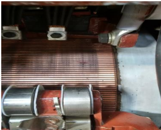
Photo 4 & 5: Commutators without V- grooving
