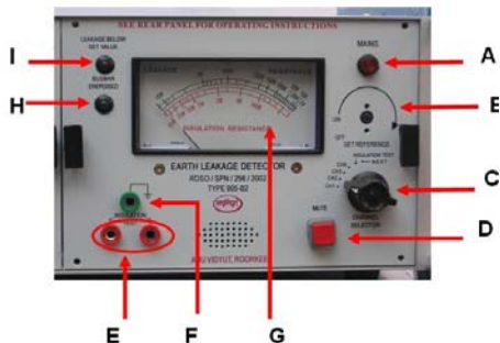
Fig.3: Controls & indications of Main module
