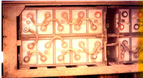
Figure 2.2 Fitment of battery in the coach
