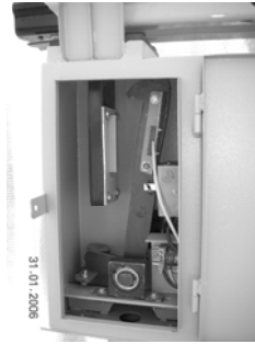
Fig.3(b) Unlocking by energizing solenoid.
