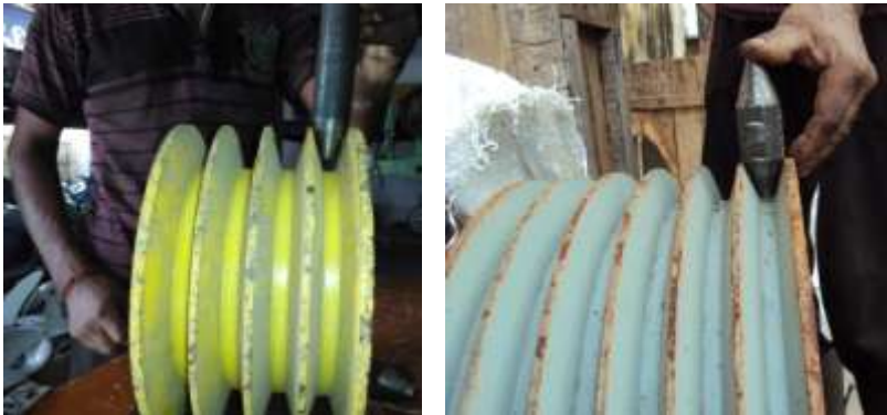
Figure 3.4. Groove checking of Alternator pulley and axle pulley
