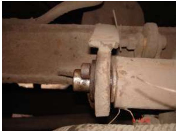
Figure 3.3. Washer put in the gap between suspension bracket
