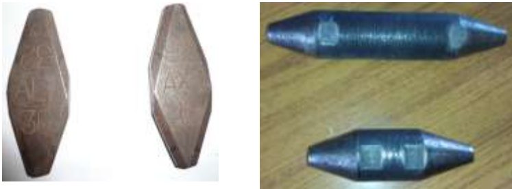
Figure 2.5. Gauge for checking groove angle of Alternator and Axle pulley
