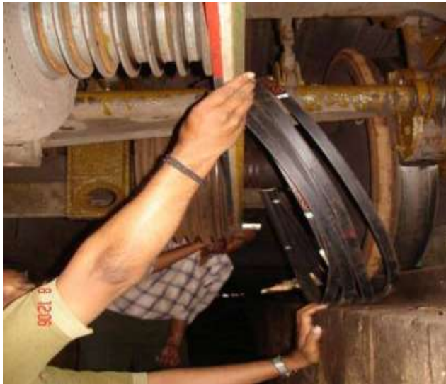
Figure 3.1. Alignment checking of alternator and axle pulleys using metal bar
