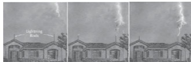
**Graphic shows (1) downward leader descending from cloud (left picture); (2) upward streamers emerging from lightning rods and tree (middle picture); and (3) leader-streamer connection (right picture). Source: Uman, M. A. and Rakov, V. A., “A Critical Review of Nonconventional Approaches to Lightning Protection”, Bulletin of the American Meteorological Society, December**
