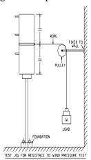
CLS Multiunit housing and Route housing fitted with all arms, as the case may be, should be fixed on a 3 m tall signal post and a load W to be applied to the centre of the housing. Load should be applied starting from 25 kg and thereafter gradually increasing in steps of 5 kg or less till it attains the value as given below.
