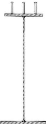
STUDS (IF ANY) TO BE WELDED AFTER COMPLETE FABRICATION OF GIRDER AT WORKSHOP OR SITE AS DESIRED
