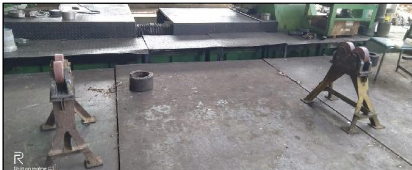
Arrangement for holding of axle before assembly
