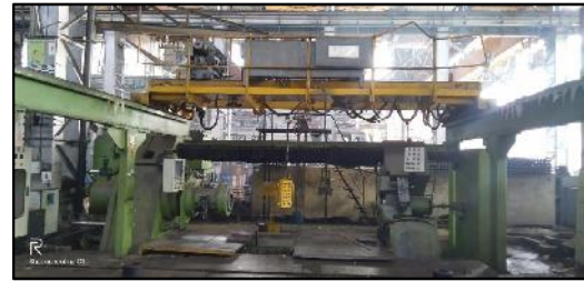
Old CNC Wheel Press Machine DoC: 27.04.2002 Make: M/s Electropneumatic & Hydraulics (India) Pvt. Ltd. Pune
