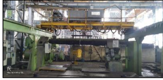
Old CNC Wheel Press Machine DoC: 14.09.2013 Make: M/s Electropneumatic & Hydraulics (India) Pvt. Ltd. Pune
