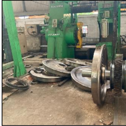
Improper Stacking of wheels
