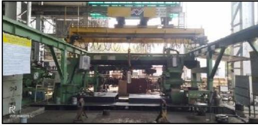
New CNC Wheel Press Machine DoC: 24.12.20 Make: M/s Electropneumatic & Hydraulics (India) Pvt. Ltd. Pune
