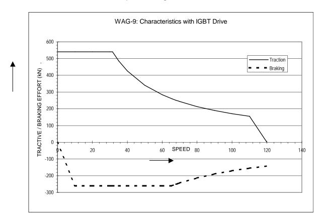
The maximum starting tractive effort generated by the propulsion system should be 540 kN under dry rail conditions.
