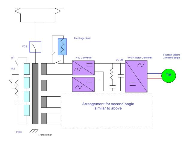
DC link shall be designed to ensure power balance between the input and output at the specified operating range. The capacitors used shall be either oil impregnated or dry type. The tenderer shall elucidate the reasons for using the type proposed, giving merits. Traction converter must have its own pre-charging arrangement of the dc link. It should be possible to earth the dc link for maintenance, which shall be interlocked with locomotive power system.
