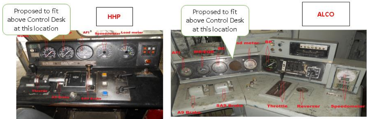
Proposed location of KAVACH in single cab HHP Locos (Long-Hood side) (Fig. 26)
