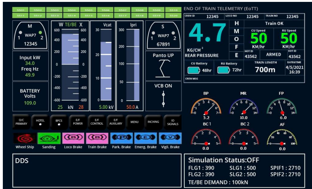
Primary Display with DPWCS Enabled for 3-Phase Locomotive (DDU-1) (Fig.-14)
