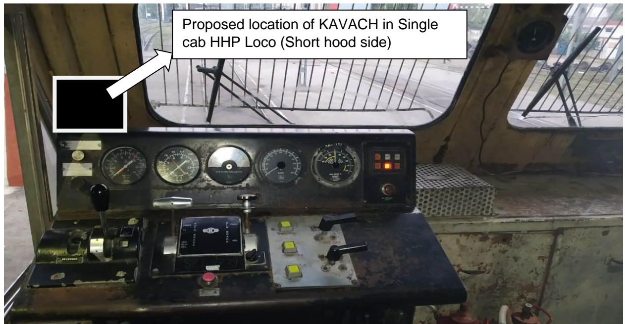
Proposed location of KAVACH in single cab HHP Loco (Short-Hood side) (Fig.-27)
