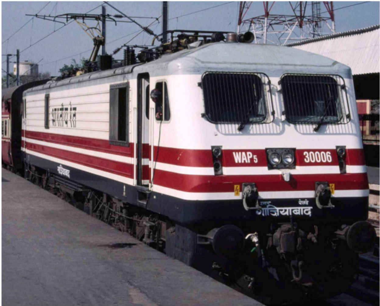
Three Phase Electric Locomotive-WAP5
