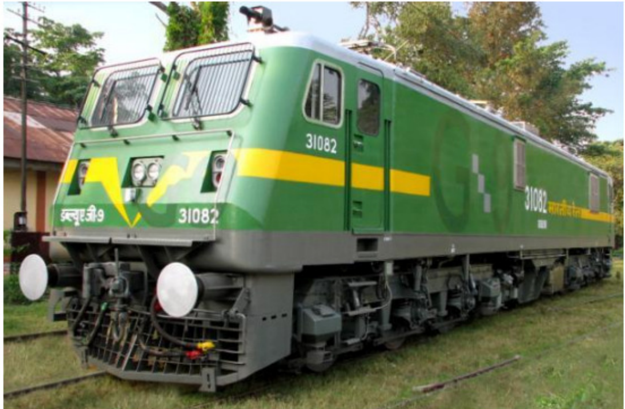
Three Phase Electric Locomotive-WAG9
