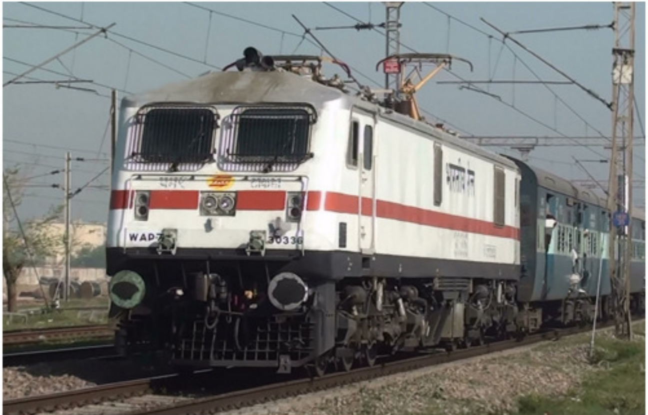
Three Phase Electric Locomotive-WAP7
