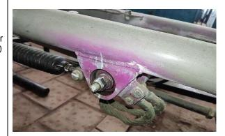
M12X1.75MM Pitch through stud fitted with double locknut
