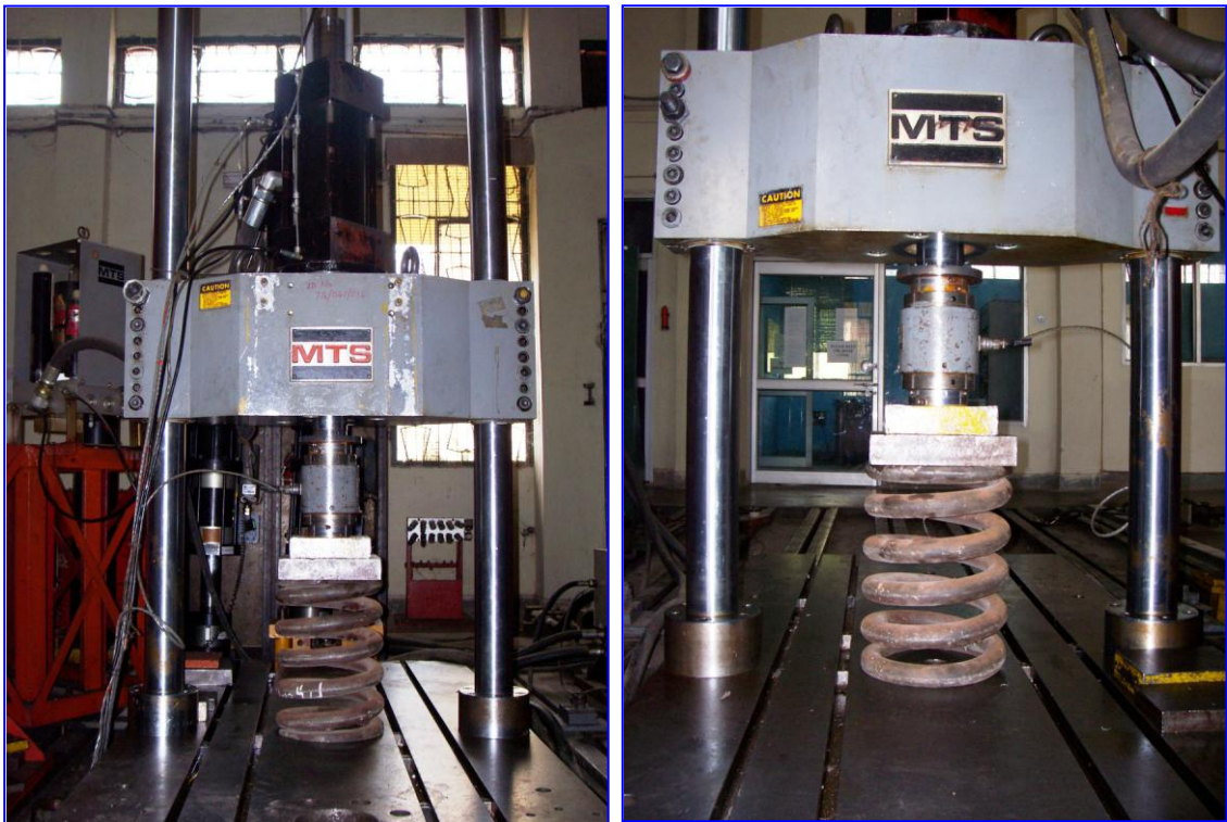
Fatigue Testing Setup for Locomotive Springs
