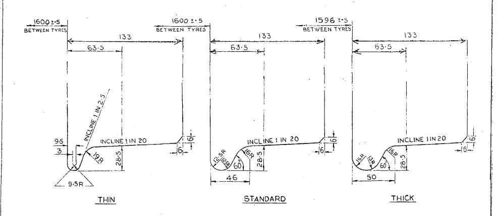
FINISHED IRS TYRE PROFILES FOR 1676 mm GAUGE LOCOS
