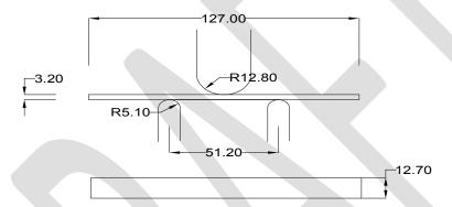
Size of the test specimen will be 127mm length, 3.2 mm depth and 12.7mm width. The specimen is deflected until rupture occurs in the outer surface of the test specimen or until a maximum strain of 5% (maximum deflection 6.8 mm) is reached whichever occurs first.
