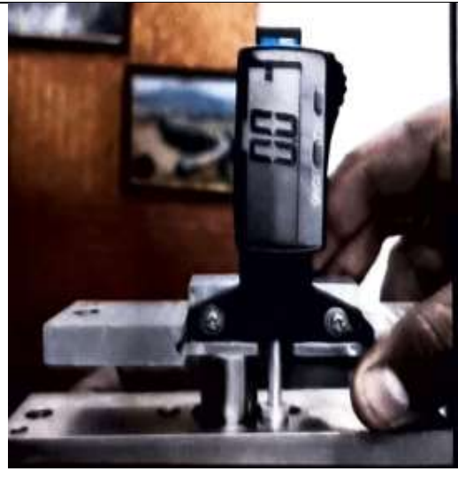
Figure – 13: Set the tip of sensor as reference.
