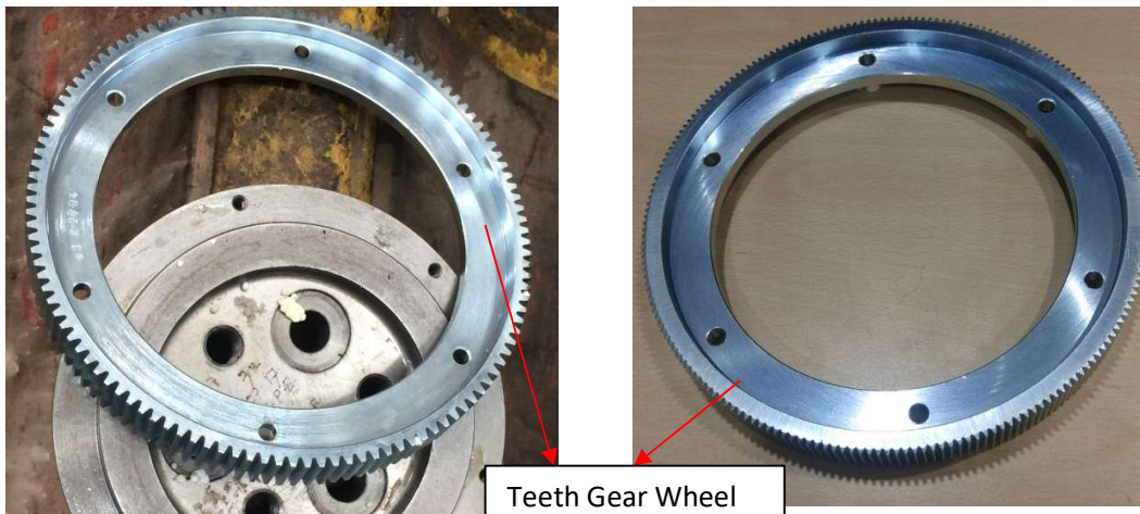
120 Teeth gear wheel used by all manufacturer except M/s BTIPL
