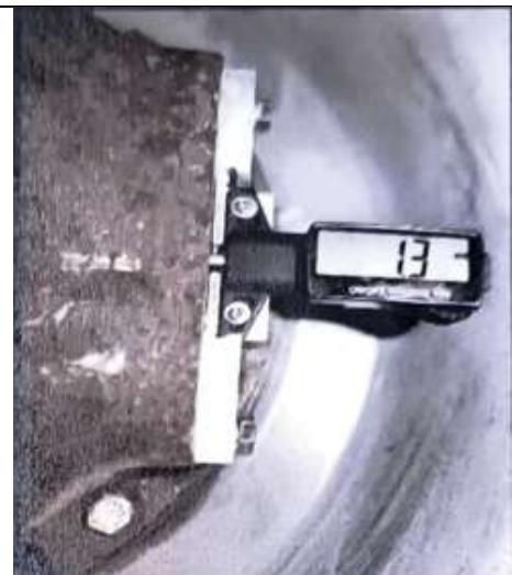
Figure – 15: Reading shown on screen is 'Measured Air Gap'.
