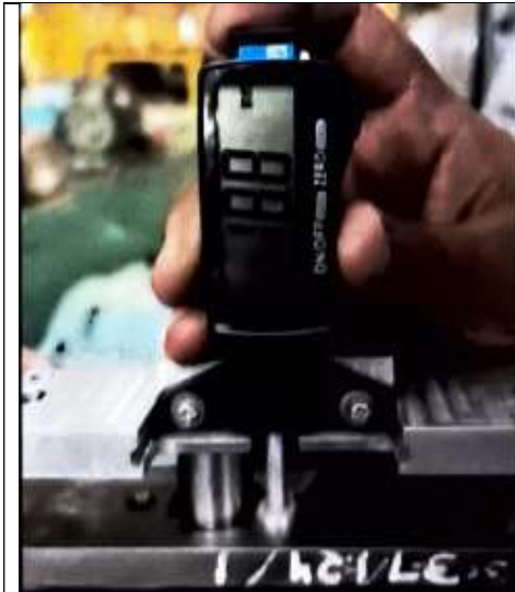
Figure – 12: Measuring the speed sensor probe.
