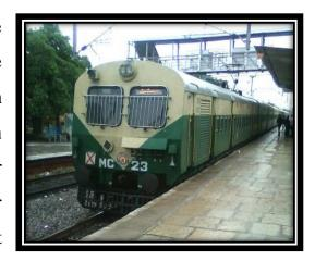
is widely used for suburban services. During the visit of MEMU train no. 04296; it was observed that the train has three units and each basic unit consists of one driving motor coach and three trailer coaches.
