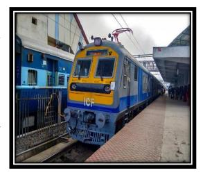
consists of three coaches in which one motor car and two trailer cars are connected with each other. Each rake of this train is a combination of three, four or five of its unit. These trains are popular due to its fast acceleration, deceleration and pollution-free operation.
