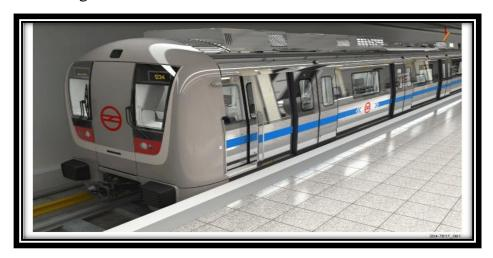
The train Formation consists of- Driving Trailer Car, Motor Car and Trailer Car. Each of these cars have different carrying capacity of passengers-
