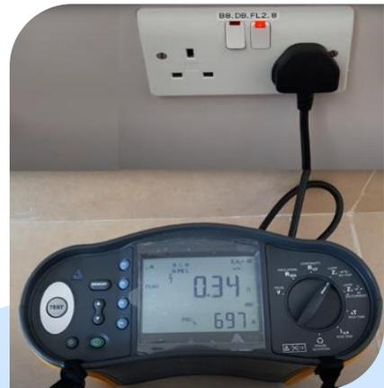
Measurement of Fault loop Impedance using fault loop impedance tester
