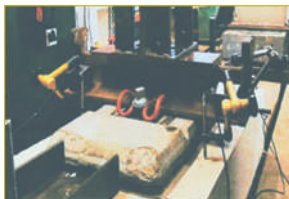
Fig.-39: Test rig for the determination of the vertical stiffness of the system
