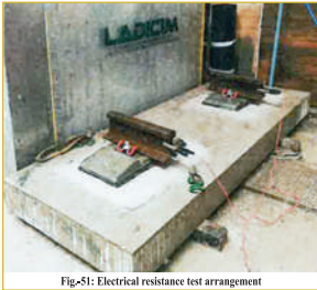
Fig-51: Electrical resistance test arrangement
