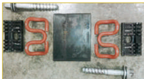
Fig. -48: Fastening components after all mechanical test
