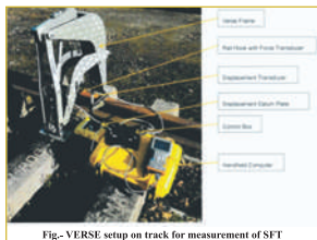
Fig.- VERSE setup on track for measurement of SFT
