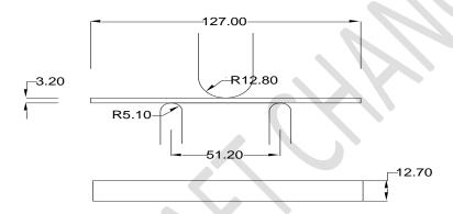
Size of the test specimen will be 127mm length, 3.2 mm depth and 12.7mm width. The specimen is deflected until rupture occurs in the outer surface of the test specimen or until a maximum strain of 5% (maximum deflection 6.8 mm) is reached whichever occurs first.
