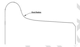
18.7 **Root Thickness (RT):** The thickness of flange horizontally measured below 22 mm from flange apex is known as root thickness. When the same is reduced to less than prescribed limit the defect is called a root wear.
