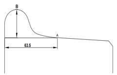
18.6 **Root Radius:** The radius of the root curve reduces to less than 13 mm, the condition is called worn root. It is the radius of root of flange of a wheel. If the radius of the root curve reduces to less than 13 mm, the condition is called worn root. (Note: For the coordinates of center for corresponding arc radius DRG No. SK.DL.-2561, SKETCH-91146 & CONT-9404/S-13 of this specification may be referred for respective wheel)
