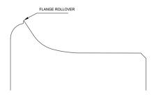
18.10 **Tread rollover:** The displacement of the metal from the rolling surface to the chamfer and then to the outer edge of the rim. The distance from the outer edge of the rim to the most protruding part.
