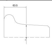
18.2 **Wheel gauge**: Wheel gauge is the back-to-back distance between the inner surfaces of the wheels in a wheelset. No profile defect is associated with this measurement.
