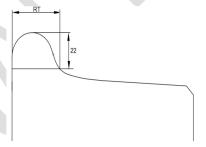
18.8 **Tread Hollow (TH):** When the center of the wheel tread is worn below the level of the end of the tread the defect is called hollow tread. It is the vertical distance between end of tread and center of tread.
