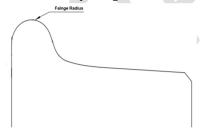
18.4 **Flange Thickness (FT):** The thickness of flange horizontally measured below 13 mm from flange apex is known as flange thickness. When same is reduce to less than prescribed limit the defect is called a thin flange.
