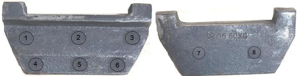
Figure-1- Reference area for checking coating thickness on Galvanized Metal Liner
