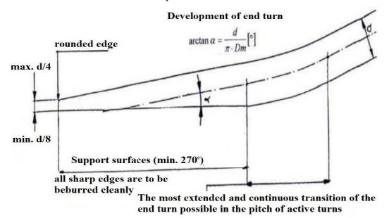
7.2.3 Proper care should be taken during the formation of ends of the springs. Correct ends formation shall be ensured as shown in Figure below:
