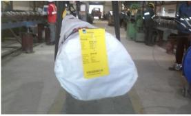
Weigh the bundles and identify them with tags detailing the size, grade, length, heat no., P.O. no., weight etc. record the readings in the Internal inspection format/job card with
