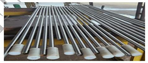
6.3.3 Sample check of bars/rods should be carried out for checking of rusting and straightness of bars/rods before manufacturing process. The stacking of bars/rods may be done according to the production schedule. The long storage of bars/rods should be avoided as it leads to loss of straightness and initiation of rusting.
