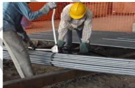
Put at least four straps on the bundle with strapping clips. Put two straps each at approximately 600 mm from the end of both sides of bundle. The other two straps shall be placed by proper spacing from the end straps. Tight the straps by a manual/pneumatic tensioner and tight the clip to clamp the bundle.
