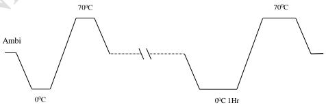
The rate of rise /fall of temperature shall be minimum 10°C/minute.
