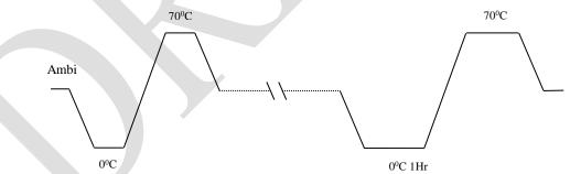
The rate of rise /fall of temperature shall be minimum 10°C/minute.
