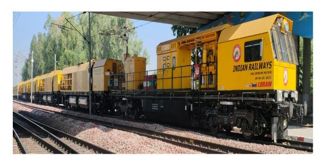
Inspection Check List of Rail Grinding Machine (RGM-96 Stone)
