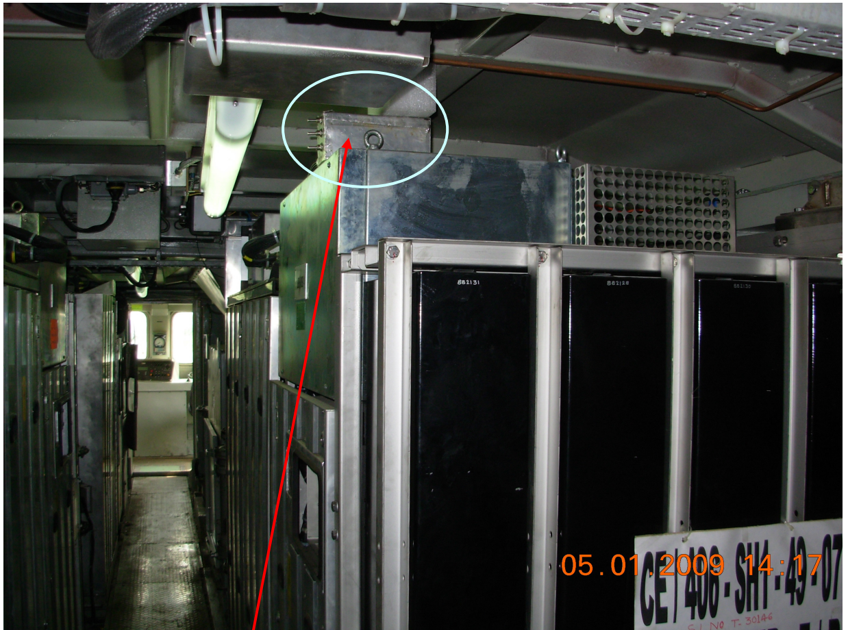
Location of Speed change over switch mounted on SR-1
