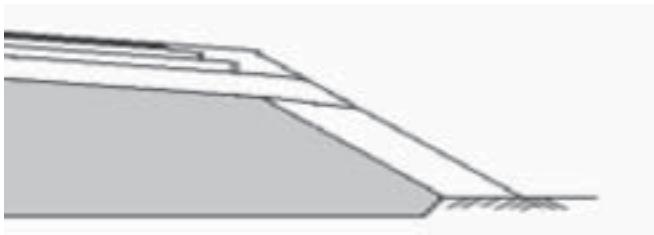
**Fig. 1 : Excavation of earth from alignment of embankment for providing side cover**
