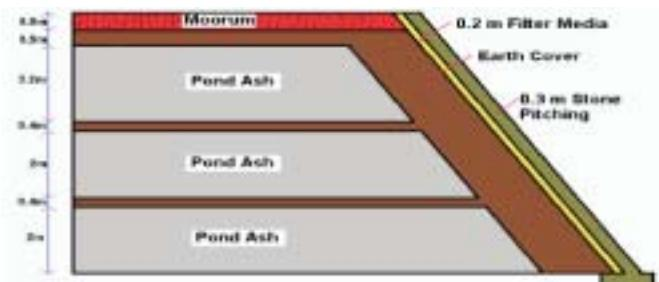
**Fig. 2: Cross-section of fly ash embankment**
