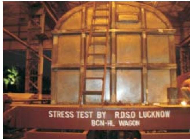
**Fig.12:End view of loaded BCNHL wagon**
