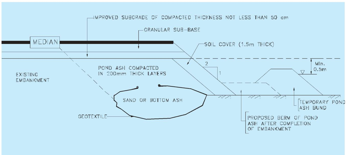
Fig. 3 : Embankment section proposed In NH-6 project
