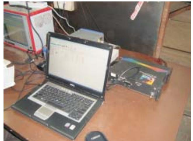
Fig.8:IOtech system (Laptop with waveView software + strain book/616)
