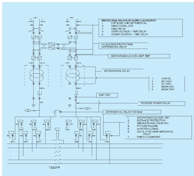
**Fig. 3 : Protection scheme for proposed 25 kV TSS**
