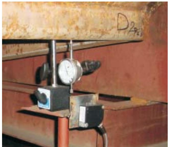
Fig.9:Magnetic base dial gauge & laser sensor in position
