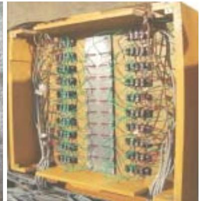
Fig.3: View of a Junction box with strain gauges fixed on dummy plate
