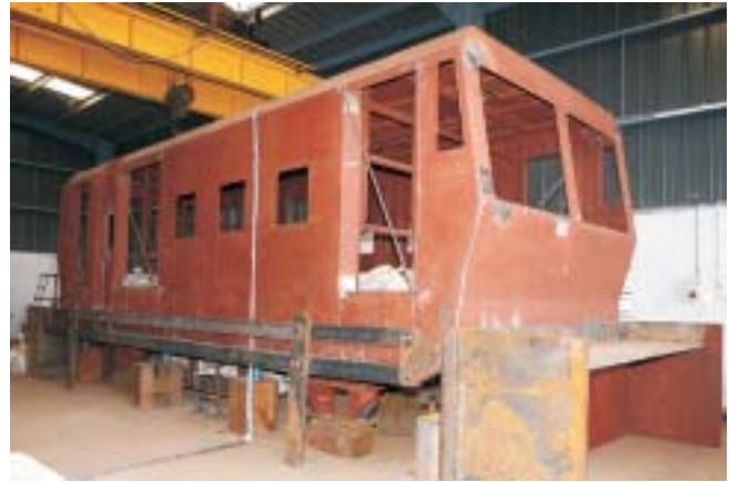
**Fig.11:View of OHE tower car wagon undergoing stress investigation tests**
