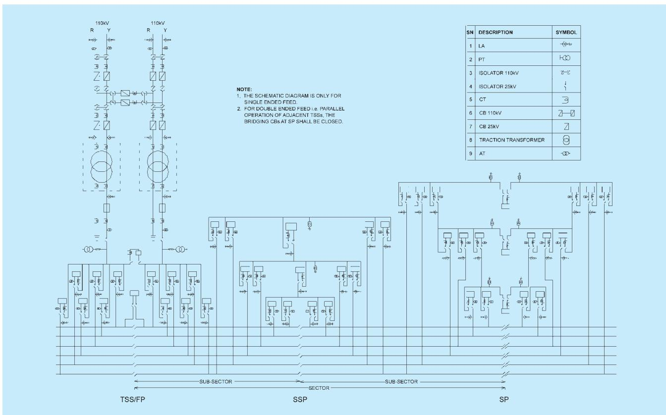
**Fig. 2 : Schematic diagram for proposed 25 kV TSS, SSP & SP**
