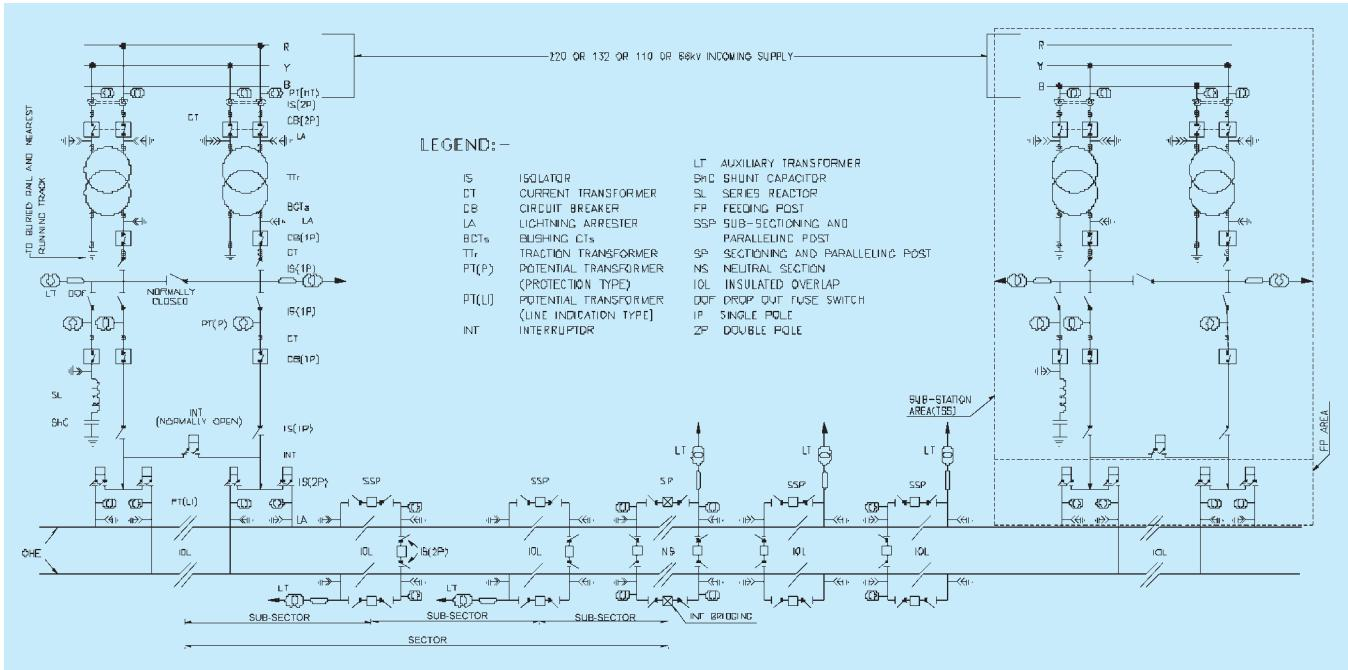
**Fig. 1 : General scheme of supply for 25 kV 50 Hz. Single phase traction system**
