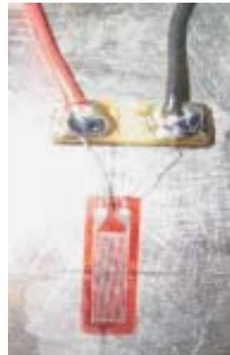
Fig.2: Enlarged View of a linear strain gauges fixed on a surface
