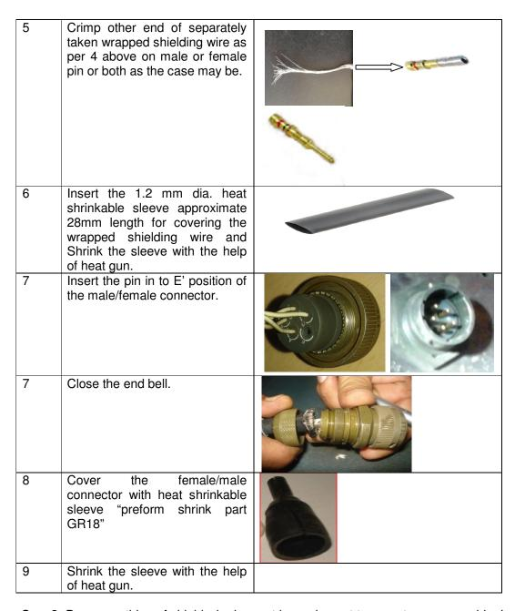
**Case2:** Proper earthing of shield wire has not been done at temperature sensor side. In order to address this deficiency, take following action: Open the temperature sensor side cable end. Check weather proper shield wire is connected to body as shown in below figure. If not, ensure following:
